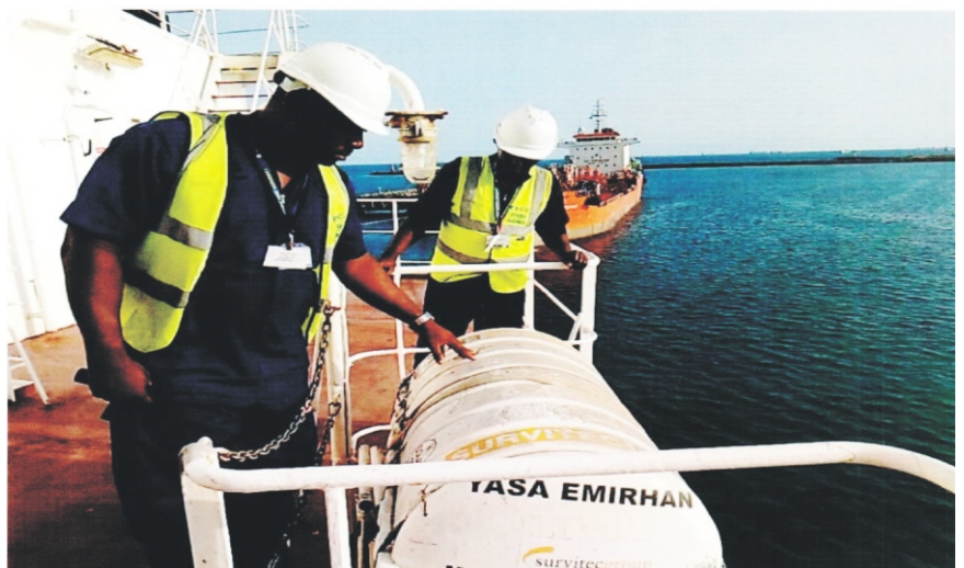
Figure 2: Checking the life raft expiring date Directorate of Maritime Affairs
