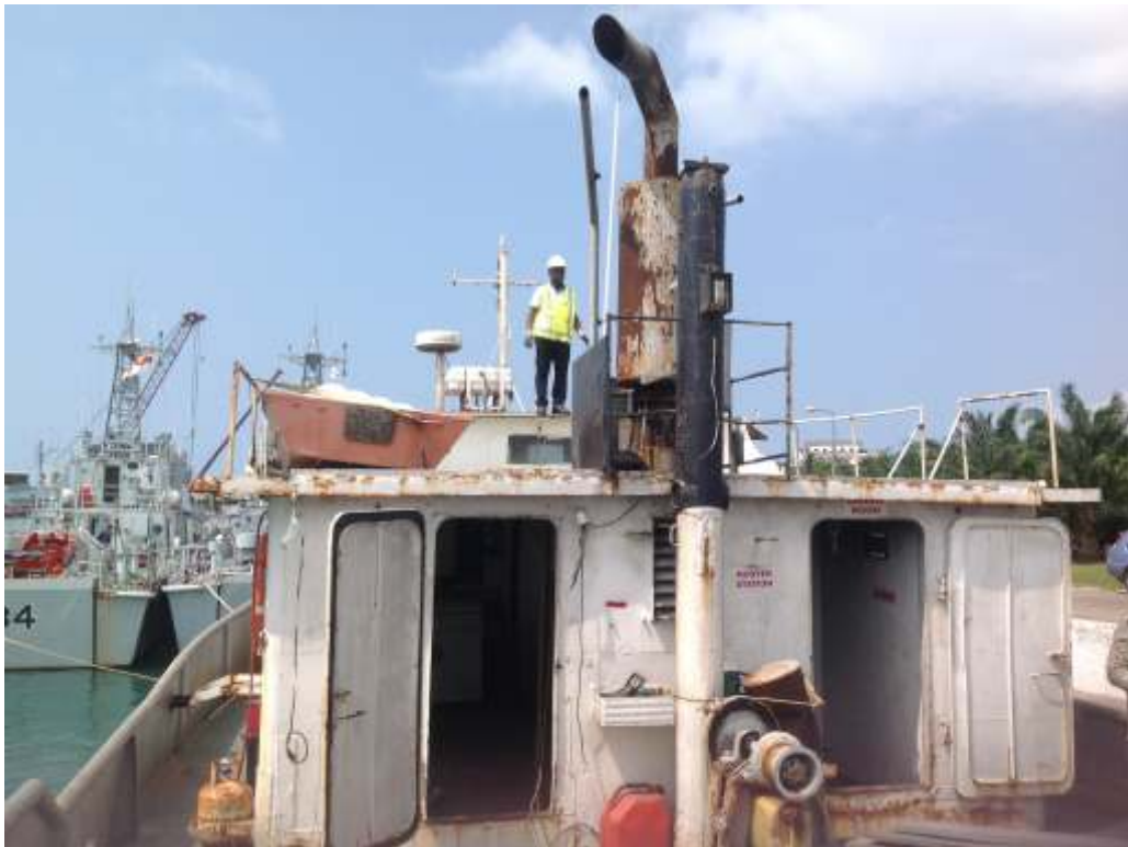
Ghana PSCO Inspecting Rusted Exhaust Funnel on Ship
