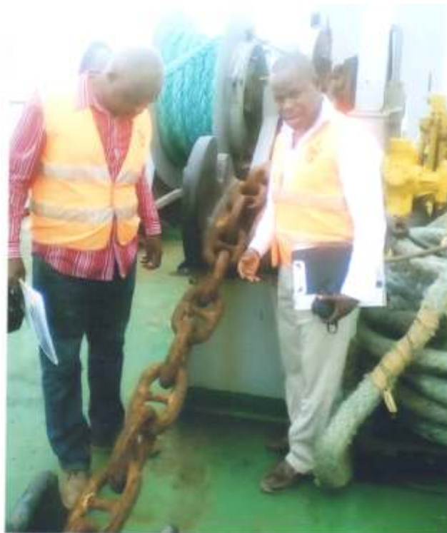
Corroded and wasted Anchor Chain
