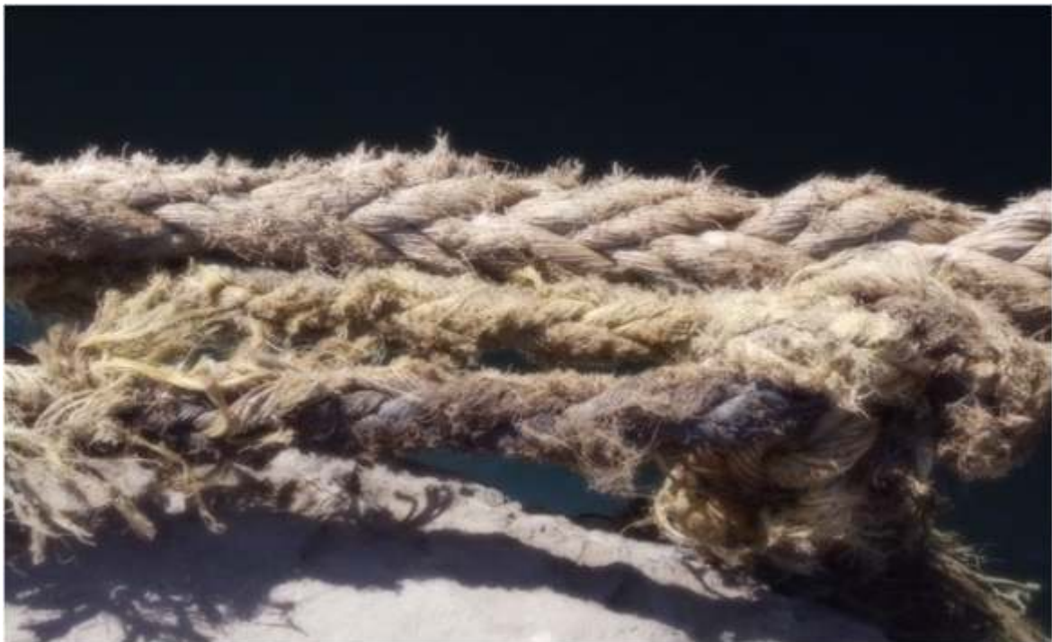
Frayed mooring line
