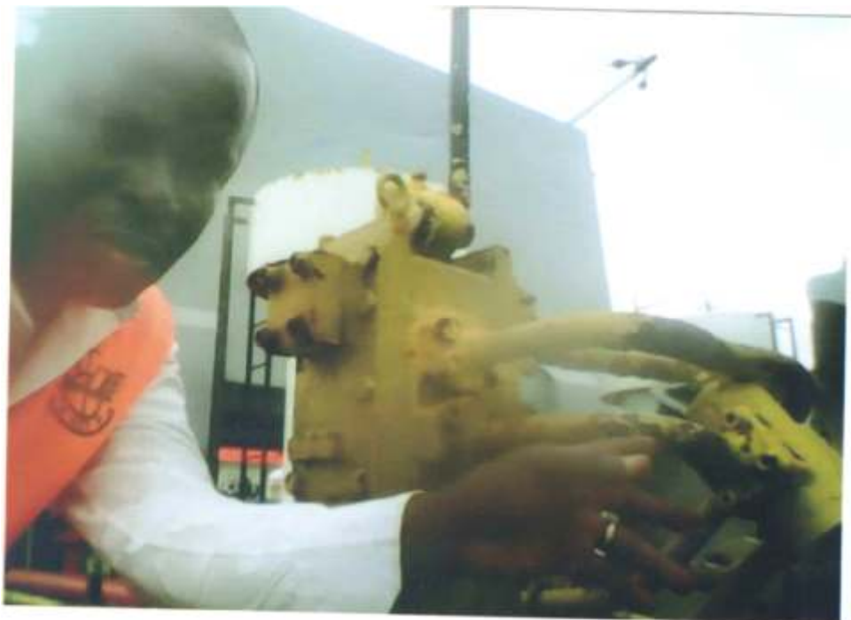
Corroded and leaking hydraulic pipe
