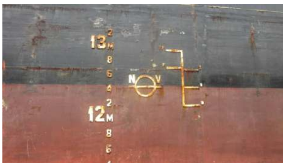
Fading and Rusting Plimsoll Mark
