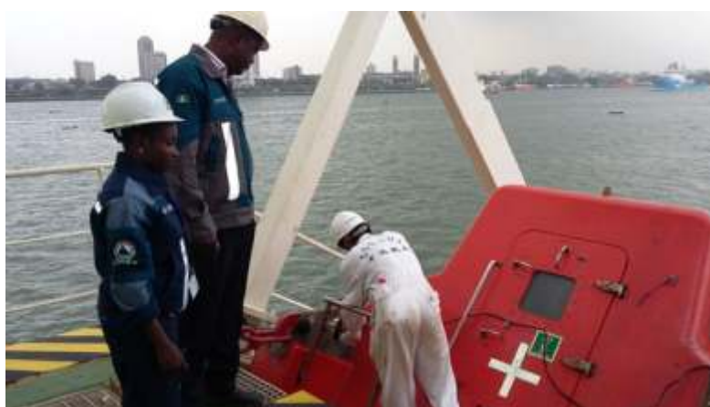
PSCOs Inspecting Free-fall Lifeboat
