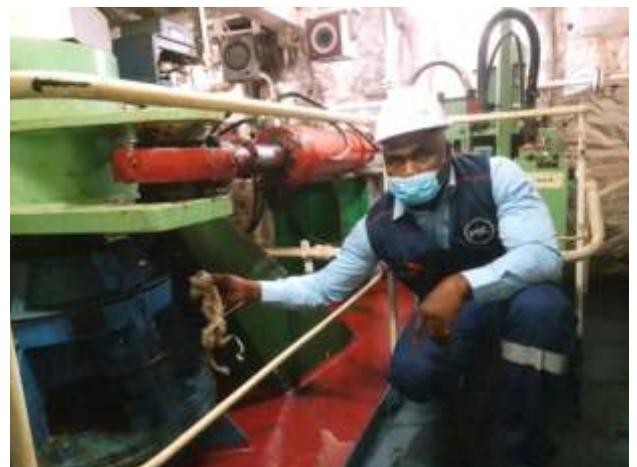
PSCO INSPECTING THE RUDDER STOCK CASING IN THE STEERING GEAR ROOM
