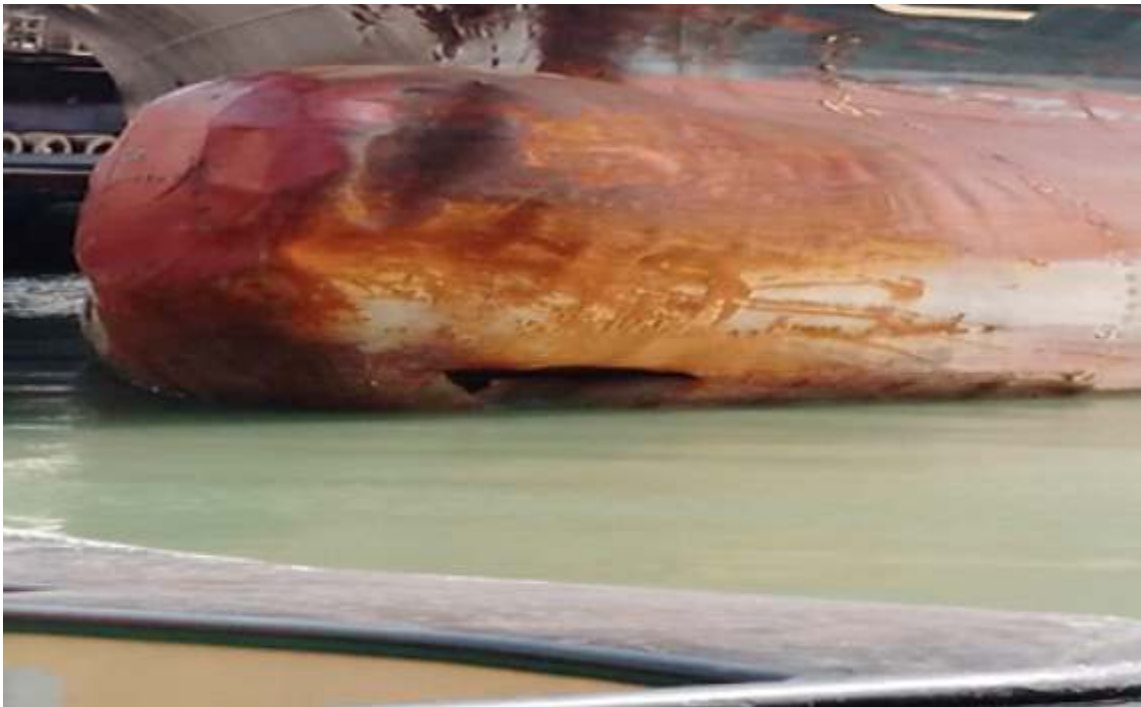
Inspection of damaged, corroded, and ruptured Bulbous Bow
