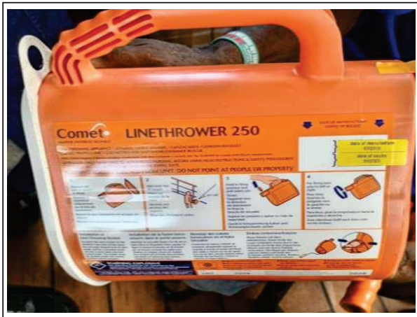
Expired line throwing equipment
